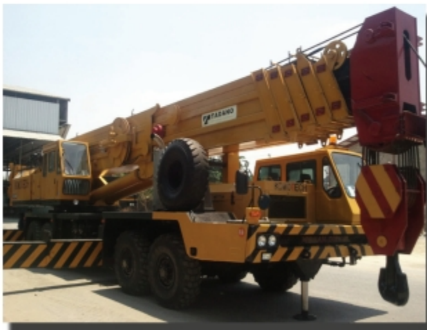
Hydraulic Crane (Tadano Crane-120 Ton)
